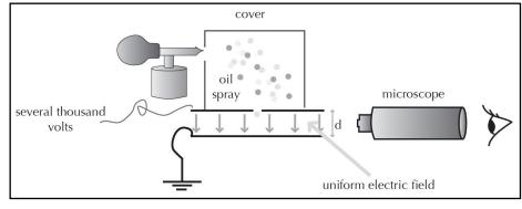
sprayed into a chamber through a nozzle. Friction in the nozzle makes some droplets become charged. The droplets fall through the chamber into the area between two metal plates. At first, the voltage is turned off. All droplets fall due to gravity. Then the voltage is turned on again. The electrical force on charged droplets works against gravity. Some drops will begin to rise. A single droplet is selected by alternately turning on and off the voltage. All uncharged droplets fall to the bottom.
